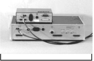
**PICOLINK -**A New Optical Fibre Link Between the AVS-47 and AVS47-IB
